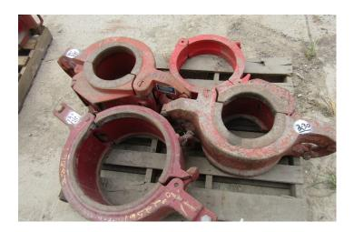
15-3/4" SD ELEVATOR, (2) 8-3/4" SD ELEVATORS, 13-1/2" SGL JT ELEVATOR
